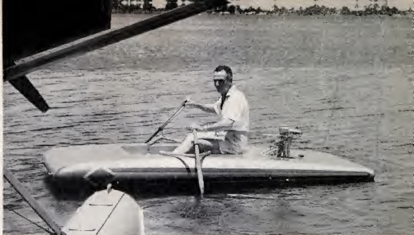
Highly maneuverable, boat weighs only 90 pounds complete with small motor and collapsible aluminum oars
